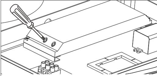
1. Unscrew both ends of the led driver cover.
