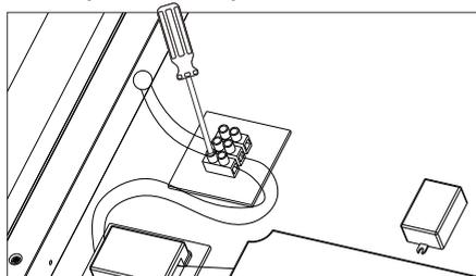
1. Loosen screw of led wire connecting terminal, remove the led wire.
