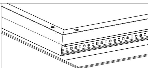
1. Tear off the PC cover around the mirror, and then tear off the led strip
