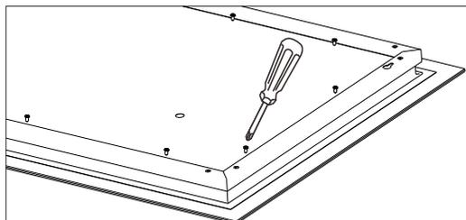
1. Unscrew the backboard and remove it.
