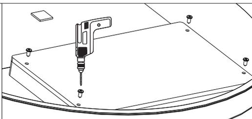
2. Unscrew the electrical box and remove the cover.
